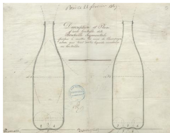
Patent No. 5175 filed on 8 March 1847 by Louis-Marie Canneaux for a type of bottle, designated a "segmental bottle", for Champagne wines and other carbonated liquids (1BB5175, INPI archives).
