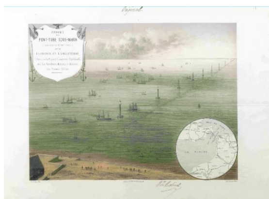
Plate filed on 1st March 1869 by Jules-Jacques Rabinel to support a patent application for "an undersea tube bridge (international railway) between France and England".
